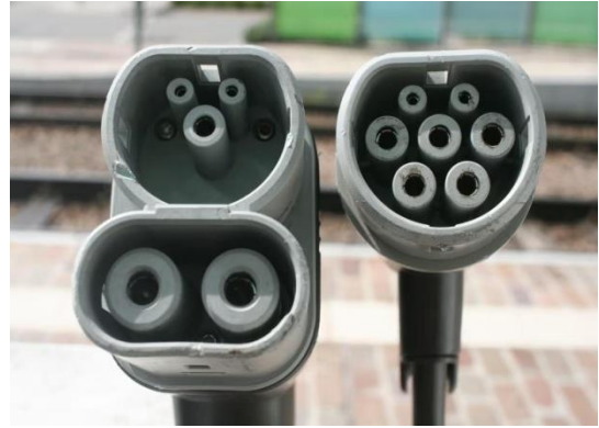
European-style combined charging system (left) and Europe-style Type 2 connector for AC charging and slow DC charging (right)
